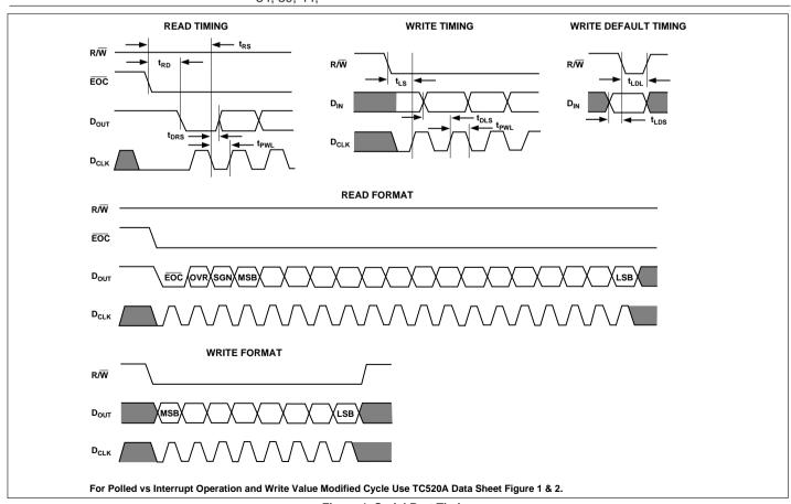
Figure 1. Serial Port Timing
