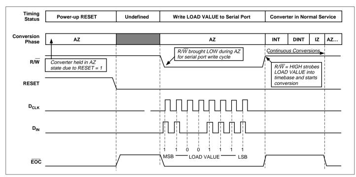
Figure 4. TC530/534 Initialization and Load Value Write Cycle
