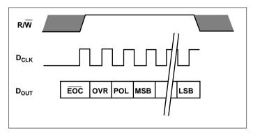
Figure 5. Serial Port Data Read Cycle
