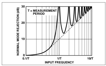
Figure 3. Integrating Converter Normal Mode Rejection
